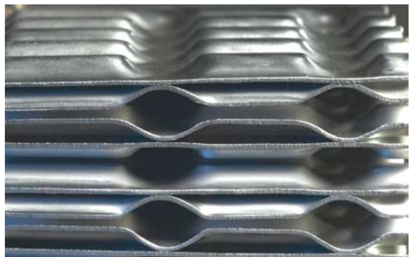
APV HYBRID platepack cut showing tube and corrugated plate sides
