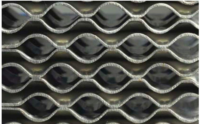
APV HYBRID platepack cut showing tube and corrugated plate sides
